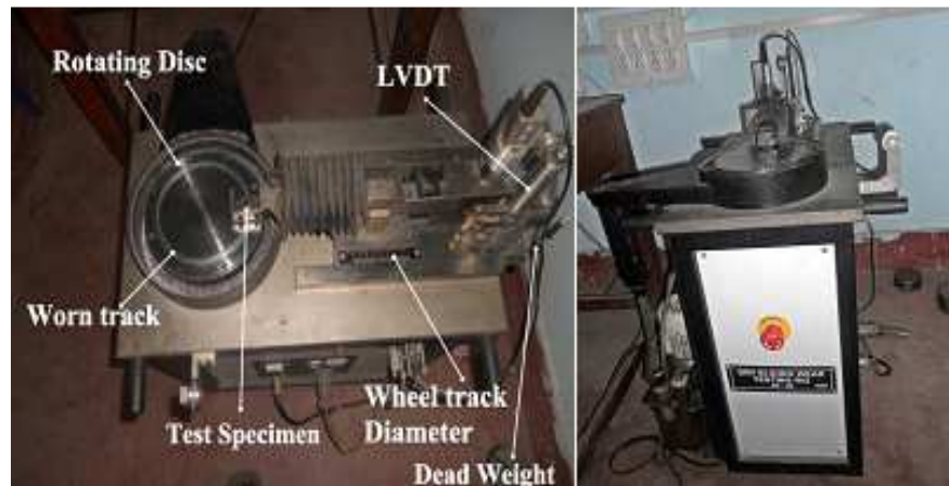
Figure 2: A Photograph View of the Pin-on-Disk Type Wear Testing Machine
