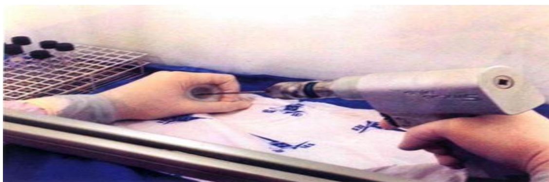
Figure 2. Collection of material from the deep layer of the polyethylene acetabular component (second phase).
