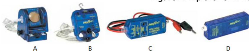
Figure 2. Xplorer GLX Sensors. A - movement sensor, B - force sensor, C - voltage/current sensor, D - absolute pressure/temperature sensor.
