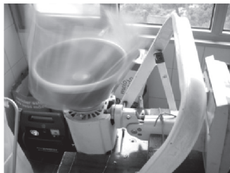
Figure 8. Physical model of artificial gravity. Because the container is rotating, the transparent protection put around it appears with a fuzzy aspect in the photo.
