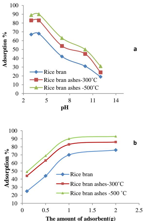
**Figure 3:** (a) The comparison of pH effects on formaldehyde removal efficiency in the three produced adsorbents (the amount of adsorbent 1 g/L, HRT of 10 hr and temperature 80°C) and (b) The comparison of dosages of three produced adsorbents on the removal efficiency (HRT of 10 hr, temperature 80°C and pH of 4)
