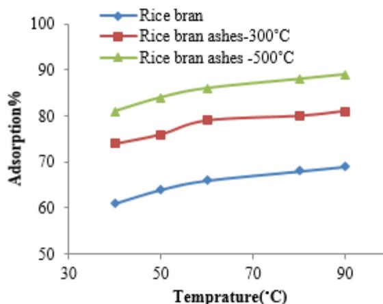
**Figure 2:** Comparison of temperature effect on the formaldehyde adsorption by three produced adsorbents (pH of 4; the amount of adsorbent 1 g/L and HRT of 10 hr)
