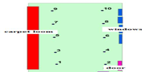
**Fig. 2:** Positions of measurement stations (1–10), carpet looms, windows, and doors in workshop II.
