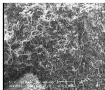
**Fig. 1:** SEM of Multi walled Carbon Nanotubes.
