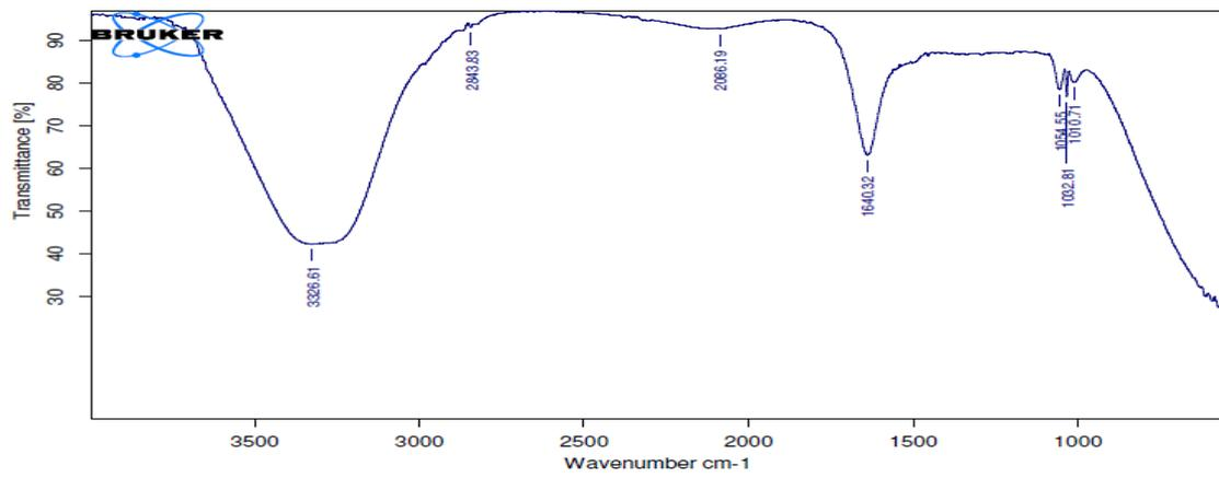
Figure 2: FTIR spectroscopy study of pure Lamivudine
