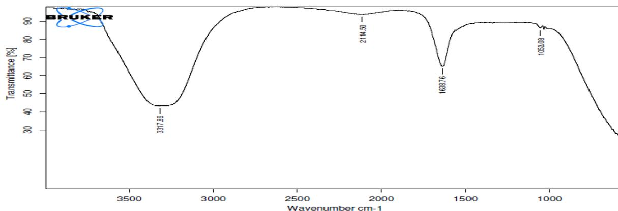
Figure 1: FTIR spectroscopy study of pure Zidovudine
