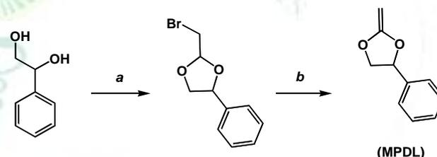
**Scheme 1:** Synthetic pathway to MPDL. Reagents: (a) DOWEX H<sup>+</sup>, bromoacetaldehyde dimethyl acetal; (b) *tert*-BuOK, Aliquat<sup>®</sup> 336, dry THF.
