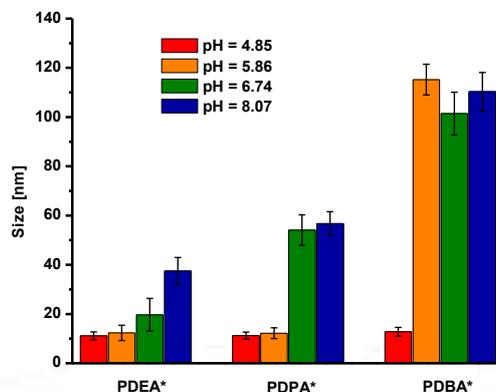
Figure 4: Particle sizes of UPS2 copolymers at difference pHs.
