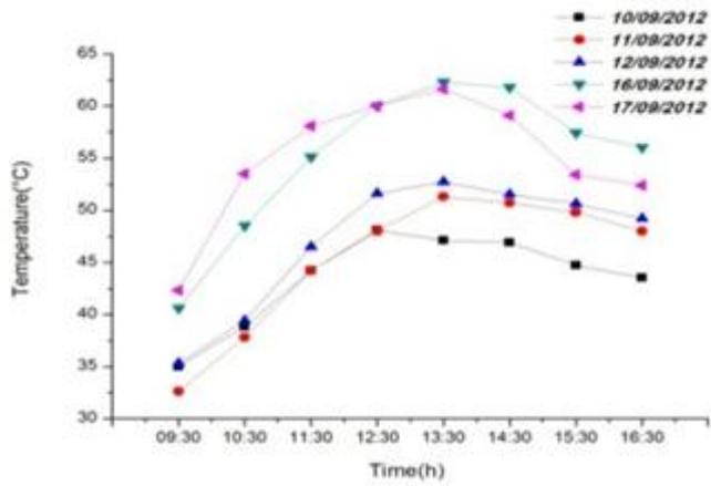
**Figure 4:** Evolution of the concrete temperatures as a function of time for different days
