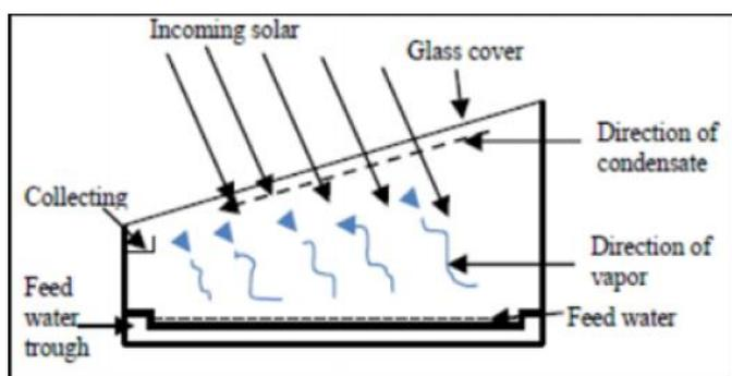
**Figure 1:** Basic operation of a conventional solar still.
