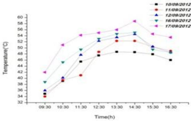
**Figure 5:** Evolution of the bitumen temperatures as a function of time for different days
