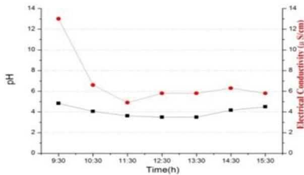
**Figure 9:** Variation of pH and conductivity versus the time. (11 sep 2012)
