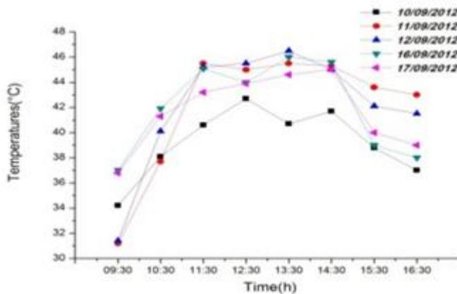
**Figure 7:** Evolution of the outer glass temperatures as a function of time for different days
