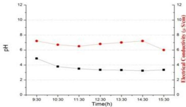
**Figure 10 :** Variation of pH and conductivity versus the time. (16 sep 2012)
