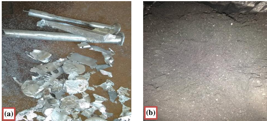
Figure 1 - (a) Cast composites samples during fettling and (b) Corn cob ash.
