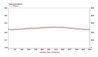
(c) In case of using the Semi-transparent photovoltaic (STPV). (Maximum and minimum annual temperature between (19.01 C° -31.45 C°).
