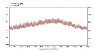
(a) In case of using the clear and simple glazing (Maximum and minimum annual temperature between 12.93C°- 47.92C°).
