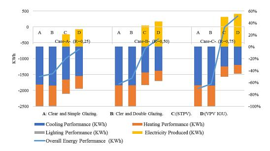
Fig.18 – Annual overall electricity benefits for different types and different Ration of system glazing (kWh).
