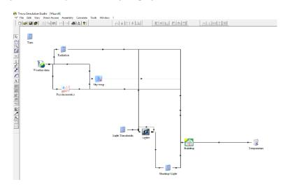
Fig. 8 – Window for assembling the project in TRNSYS simulation studio
