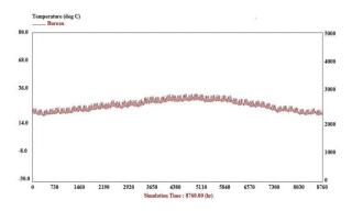
(d) In case of using the Vacuum Photovoltaic Insulated Glass Unit system (VPV IGU). (Maximum and minimum annual temperature between 20.10 C°- 33.02C°).
