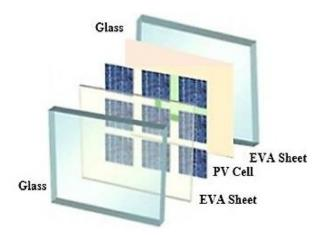
Fig. 9 – A simplified diagram of a of (STPV) structure
