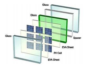
Fig. 10 –Schematic diagram of the (VPV IGU) structure.
