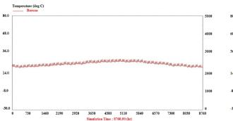
(b) In case of using the clear and double glazing (Maximum and minimum annual temperature between 19.89C° - 31.36C°).
