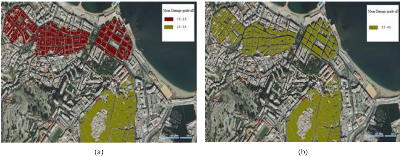
Fig.6–Mean damage grade distribution in the study area (a) for I(EMS)=VIII , (b) I(EMS)=IX .
