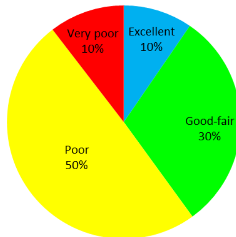
Fig. 9 – SPI classification at left bank of Souk Tleta dam foundation
