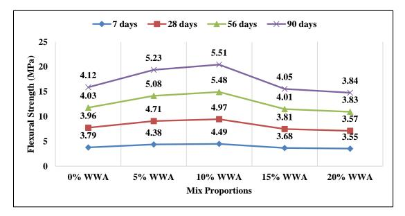
Figure 6- Flexural Strength of WWA Concrete
