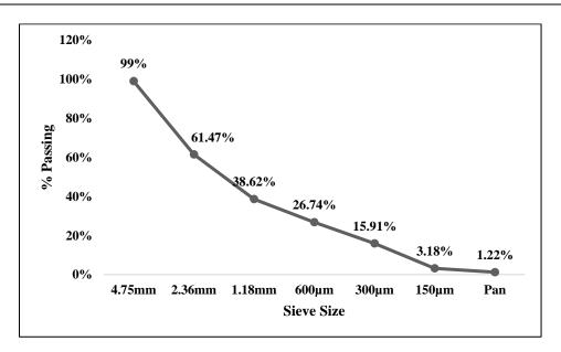
Figure 1- Gradation Curve of Fine Aggregates
