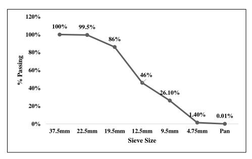
Figure 2- Gradation Curve of Coarse Aggregates
