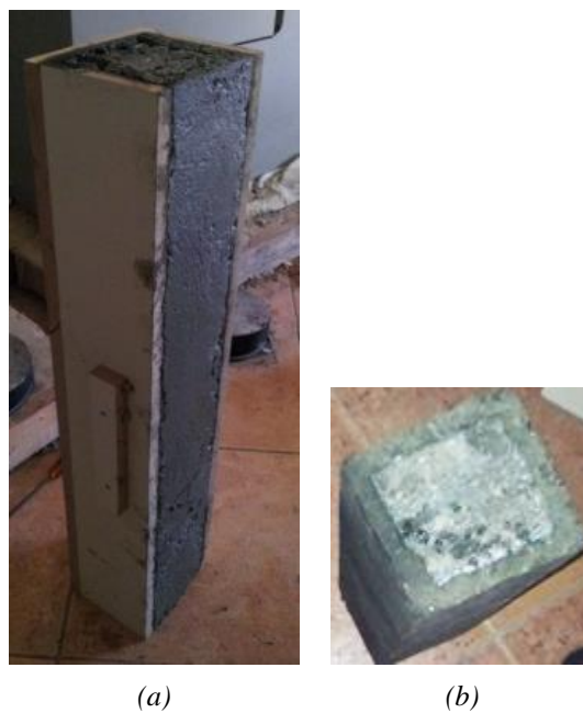
Figure 3: Column specimen after casting, (a) inside the mold, (b) outside the mold
