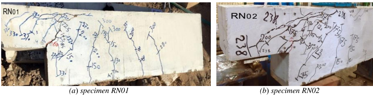
Fig. 10- Cracks Patterns for the Specimens with Reduced Reinforcement at Nib region
