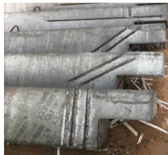
(b) Groove are cleaned and dried
