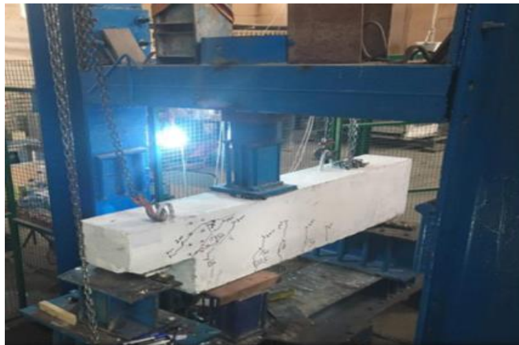
Fig. 6- Details of Strengthening of Dapped end Beams
