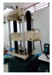
(a) Digital universal testing machine (UTM)
