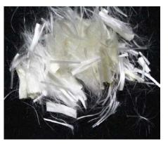
Fig. 1 – Polyvinyl Alcohol (PVA) Fibres used in the study
