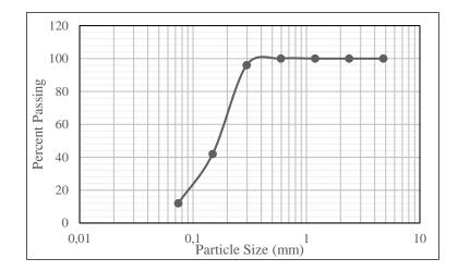
Fig. 3 – Gradation curve of fine aggregates
