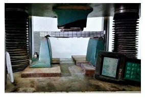
(c) Test setup of flexural strength test
