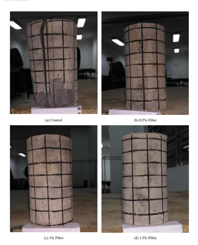
$Fig. 11-Failure\ pattern\ of\ concrete\ specimens\ after\ compression\ test$
