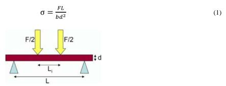
Fig. 8 - Beam under 4-point bending
