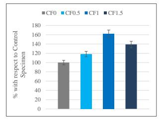
Fig. 7 – Comparison of Compressive Strength for test specimens on Day 90
