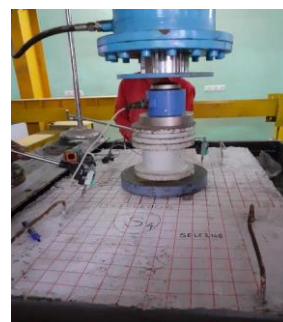
Figure 15. Loading arrangements by hydraulic jack and load cell
