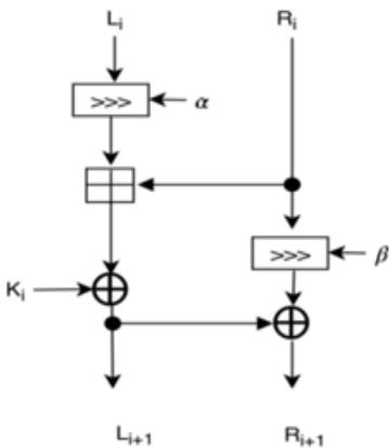
Figure. 7 Lightweight speck cipher
