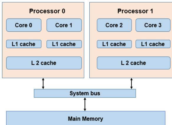
Figure. 2 Architecture of multi-core processor
