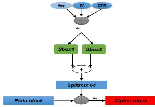
Figure. 6 Proposed lightweight encryption function
