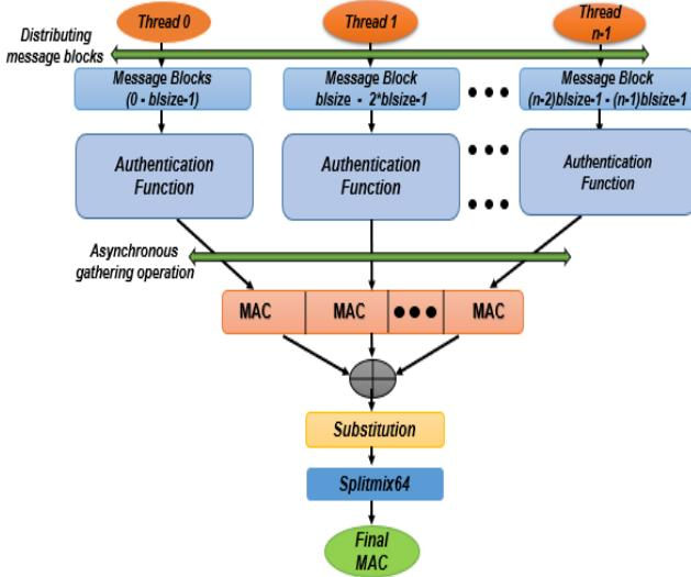
Figure. 4 The structure of the proposed parallel authentication method
