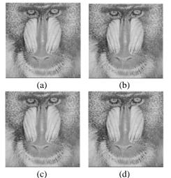
Figure. 9 The comparison results of our proposed method using grayscale in 512x512 pixels: (a) Cover image, (b) LSB, (c) Caesar-Vigenere-LSB, and (d) Caesar-Vigenere-LSB-Fibonacci
