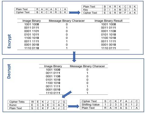
Figure. 6 Encrypt and decrypt illustration using Fibonacci
