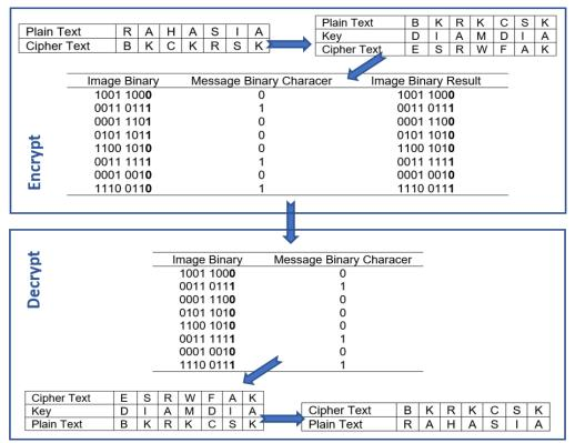
Figure. 5 Encrypt and decrypt illustration without Fibonacci
