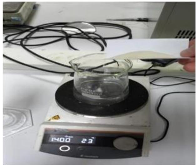
Figure 2. Preparation of chitosan solution.
