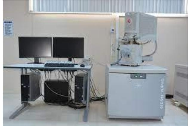
Figure 9. SEM-EDX device.
