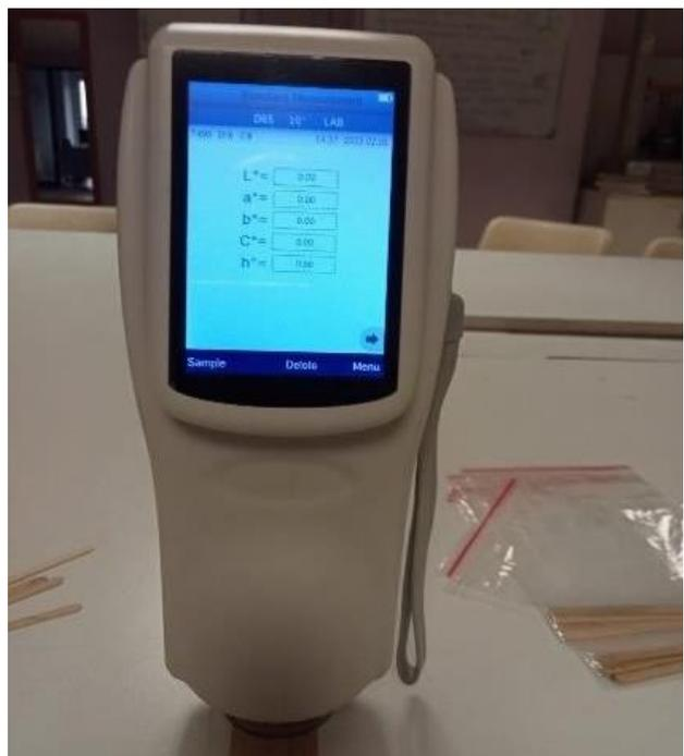
Figure 7. PCE-CSM 10 spectrophotometer device.
