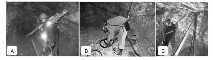
Figure 6. Postures evaluated with REBA for jackleg-drilling.
