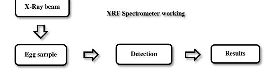
Figure 1. Working of the X-Ray fluorescent spectrometer (Epsilon-1) for the analysis of hen egg mineral contents
