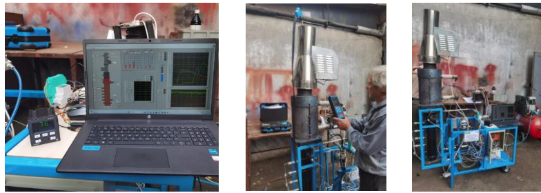
Fig. 5. Images during testing in the version with a heat exchanger located outside the drying chamber, using sensors and automatic systems
