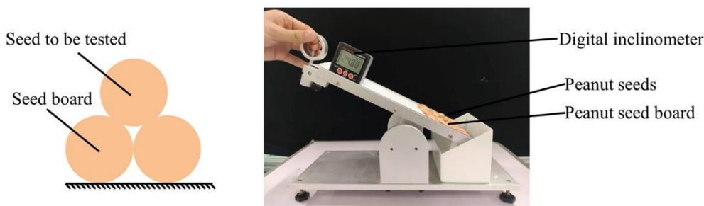
Fig. 2 - Sketch for measuring friction coefficient of peanut seeds (a) Seed board; (b) Friction coefficient testing device
