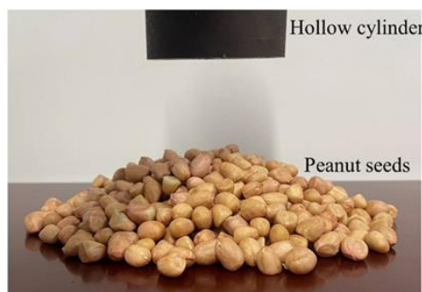
Fig. 3 - Angle of repose physical test
