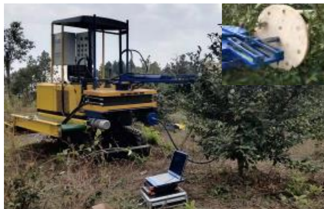
Fig. 1 - Vibrating camellia fruit harvester used in the canopy experiment
