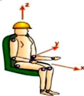
Fig.1 - The ortogonal measuring directions that effect driver WBW, (Vlăduț V. et al, 2021)
