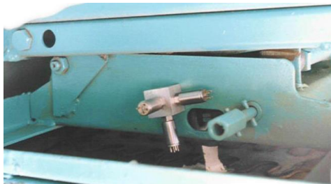
Fig. 2 - Transducers mounted on the combine seat
