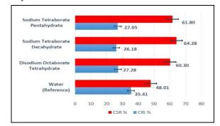
Figure 5. % CSR and % CRI values of solutions prepared using different boron products with a concentration of 5 g/l and water-quenched coke samples.
