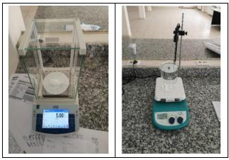
Figure 1. Preparation of solutions; weighing on precision balance and mixing on magnetic stirrer with heater.
