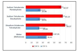
Figure 6. % CSR and % CRI values of solutions prepared using different boron products with a concentration of 7 g/l and water-quenched coke samples.
