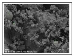
Figure 10. Three different EDS points of coke sample quenched with 7 g/l Disodium Octaborate Tetrahydrate solution.
