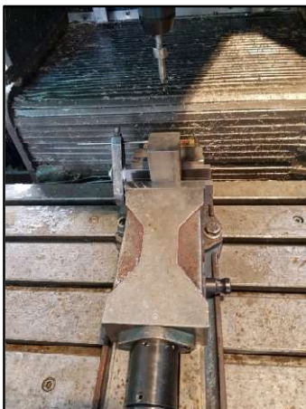
Figure 14. Clamping of work piece
