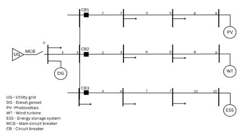
Figure 5. Microgrid Testbed
