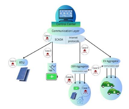
Figure 2. High Level Communication Between a Utility and DERs with Identified Points of Cyber-Attacks
