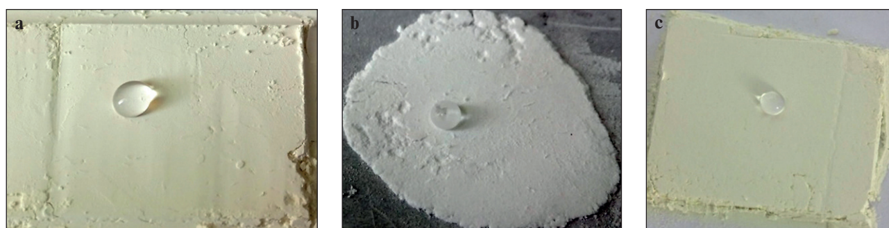
Fig. 7. Image of water droplets on pressed surfaces consisting of: a – nanosulfur; b – calcium carbonate nanopowder; c – S and CaCO 3 nanocomposite
