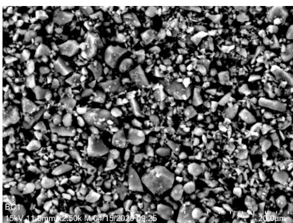
Figure 1 – Microscopic image (left) and EDS-spectrum (right) of Calorsil material. In the EDS-spectrum the chemical elements related to the signals are indicated
