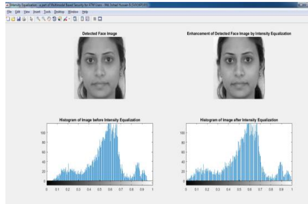
Figure. 9 Gray scale image versus enhanced gray scale image with Intensity equalization shown with their respective histograms (with same shape)
