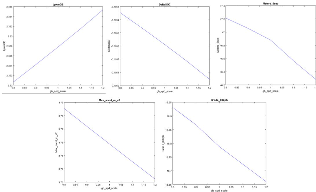
Fig.10 Parametric study considering a single variable (gb\_spd\_scale). LpkmGE – gasoline equivalent in liter/km; DeltaSOC- variation of the SOC; Meters\_5sec – distance in 5 secons, in meters; Max\_accel\_m\_s2 – maximum acceleration (m/s<sup>2</sup>); Grade\_89kph – gradeability at 89 km/h
