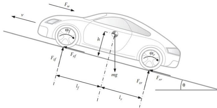
Fig. 1. Longitudinal forces acting on a vehicle [5]
