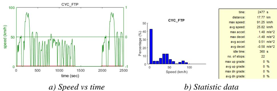
Fig. 6 FTP drive cycle
