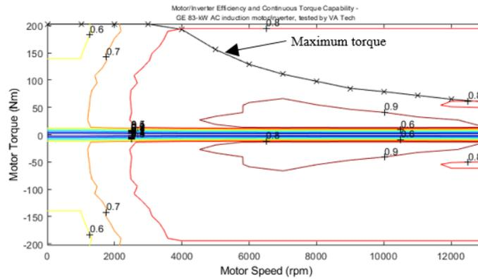
Fig. 5. Motor/inverter characteristics
