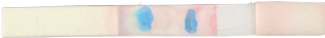
Fig. 2. The result of the developed full-strip, including the sample pad, conjugate pad, nitrocellulose membrane, and absorption pad, after being tested with 500 ng/ml SARS-CoV-2 N protein.
