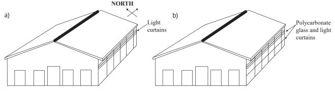
Figure 1. Easy-to-assemble premises without (a) and with (b) elements of heat insulation
