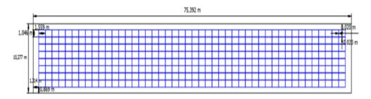
Figure 3.3. Dimensioning plan of modules.
