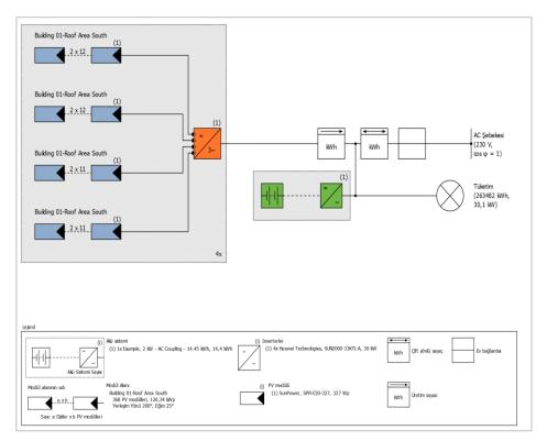
Figure 3.4. Block diagram of the designed photovoltaic system.
