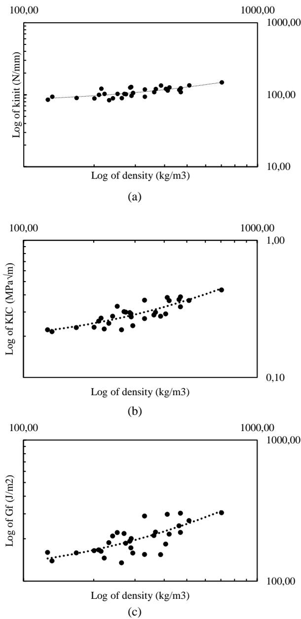
Figure 5. Log-log plots showing the relationship between (a) initial slope ( $k_{init}$ ), (b) fracture toughness ( $K_{IC}$ ), and (c) specific fracture energy ( $G_f$ ) versus density
