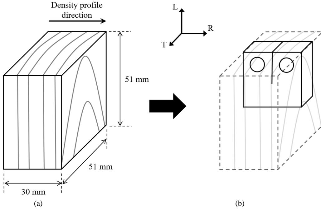
Figure 2. A typical density profile testing block configuration (a) and illustration of how a fracture test block was obtained from a measured block (b)
