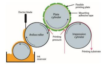
Figure 2. Flexo printing principle (Valdec et al., 2017)
