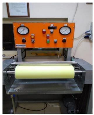
Figure 4. Size press coating machine
