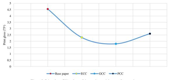
Figure 8. Print gloss (75°) values of the used materials as surface coating
