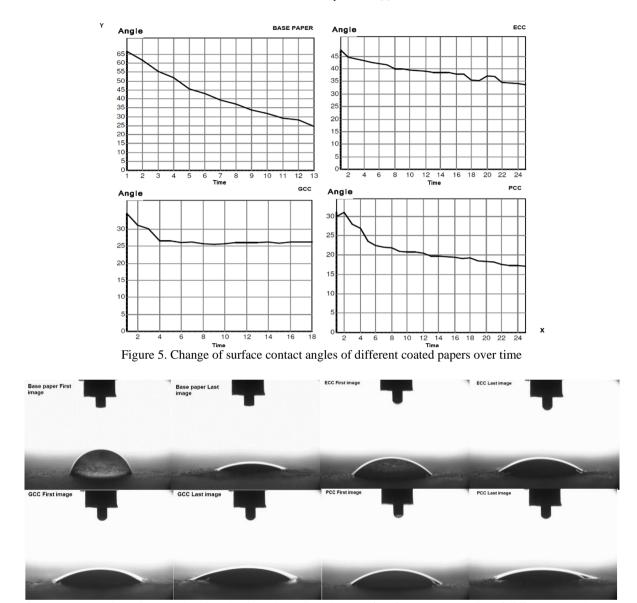
Figure 6. Drop volume images showing the time-dependent change of surface contact angles of different coated papers
