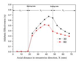
Fig. 15 Comparison of centerline adiabatic effectiveness at blowing ratio (BR) of 0.25 for different injection angles
