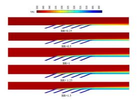
Fig. 7 Temperature slice counters on the center plane of effusion plate for different BR on XZ plane for  $\alpha{=}30o$
