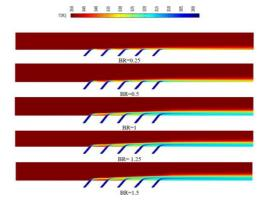
Fig.9 Temperature slice counters on the center plane of effusion plate for different BR on XZ plane for  $\alpha{=}60^\circ$
