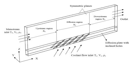
Fig. 1 Schematic of computational domain (XYZ)
