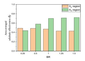
Fig. 16 Area-averaged adiabatic effectiveness ( $\bar{\eta}$ ) with blowing ratio (BR) in the effusion region (X<sub>2</sub>) and downstream region of effusion holes (X<sub>3</sub>)
