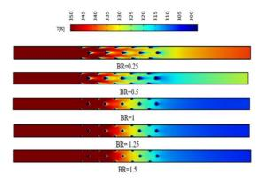
Fig.10 Temperature distribution on effusion plate surface for different BR on XY plane for  $\alpha{=}60^\circ$
