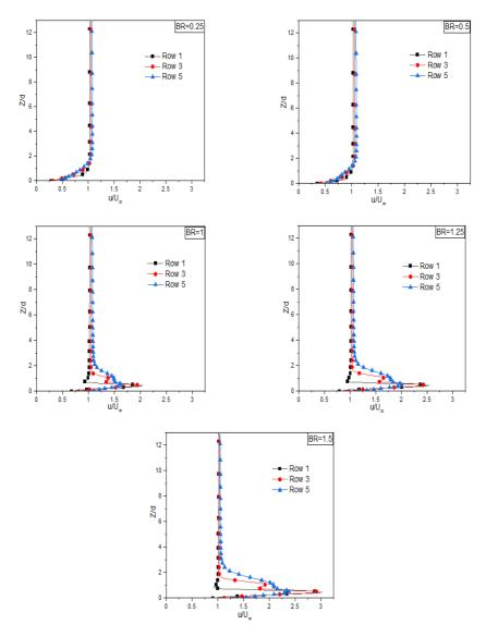
Fig.11 Velocity profiles downstream the effusion hole rows at different blowing ratios  $(\alpha=30^\circ)$
