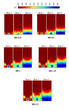
Fig. 13 Development of temperature fields on the YZ plane for different blowing ratios at  $\alpha{=}30^\circ$
