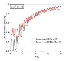
Fig. 5 Validation of experimental [23] and computational results. Note that the leading edge of first row X/S<sub>x</sub>=0 and adiabatic effectiveness is measured from rows 1 to 20
