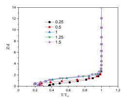
Fig. 14 Normalized Temperature boundary profiles at row 5 for  $\alpha$ =30°
