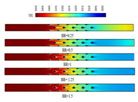
Fig.8 Temperature distribution on effusion plate surface for different BR on XY plane for  $\alpha{=}30^\circ$
