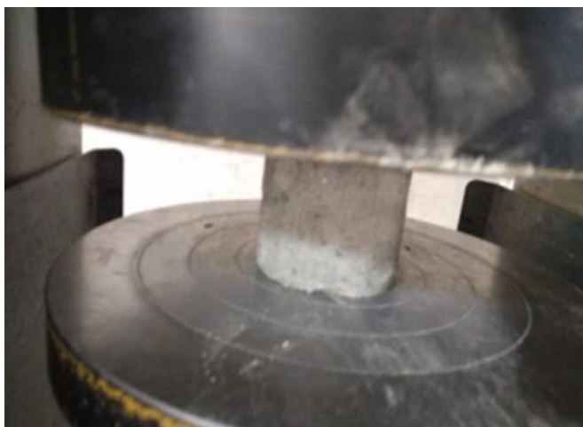
Fig. 9 Laboratory test for the concrete sample of TD_2 - 82/2
