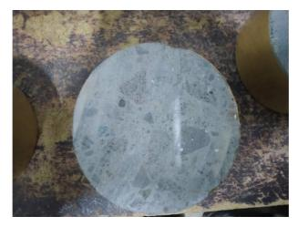
Fig. 3 Core Sample From Specimen for RCPT
