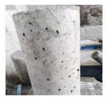
Fig. 6 Surface of Demoulded Cylindrical Specimens
