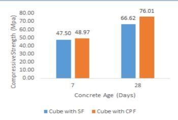
Fig. 7 Compressive Strength vs Age Test Results
