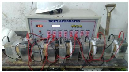
Fig. 4 RCPT Apparatus with Specimens
