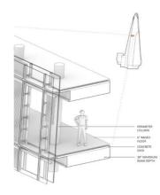
Fig. 3 The Shard Facade, Triple Glazed Detail [7]
