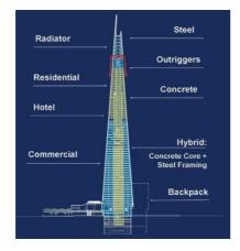
Fig. 4 Construction Technique and Usage Functions According to Shard Floors, Cambridge [9]
