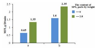
Fig. 3. MFI of modified PVC plastic at different gelation temperatures (K): a – 363; b – 403
