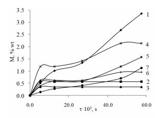
Fig. 6. Kinetics of release of plasticizer from PVC materials depending on the nature of plasticizer: 1, 5, 6 - DBP;
