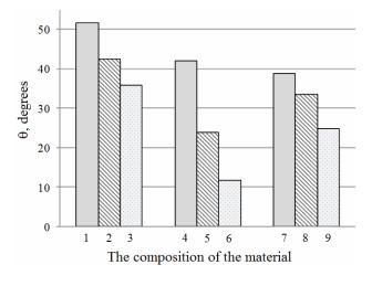
Fig. 2. The influence of the type of base on the wetting angle of the surface with plasticizers: 1-3 - DBP; 4-6 - DOP; 7, 8 - DINP; 9 - DBP:DINP= 1:1.
