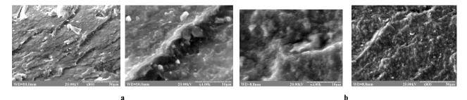
Fig. 5. SEM photos of chipped modified PVC material after gelling at 363 K (PVC:DOP=100:30): a – without modifier; b – SPS as a modifier (2.8 parts by weight)
