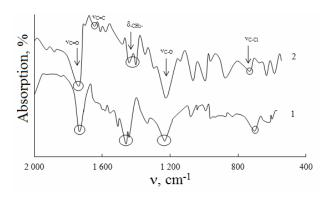
Fig. 4. FTIR spectra of the modified PVC material (PVC:DOP=100:30). Polystyrene modifier (2.8 parts by weight): 1 - SPS; 2 - HIPS
