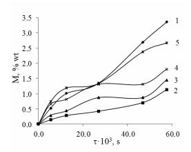
Fig. 7. Kinetics of release of DBP from PVC materials depending on its content: 1-3 - 23 wt.%; 4 - 44 wt.%; 5 - 51 wt.%; and the content of the suspension SPS: 1 - 0 wt.%; 2 - 2.1 wt.%; 3 - 3.1 wt.%; 4 - 6.6 wt.%; 5 - 7.4 wt.%
