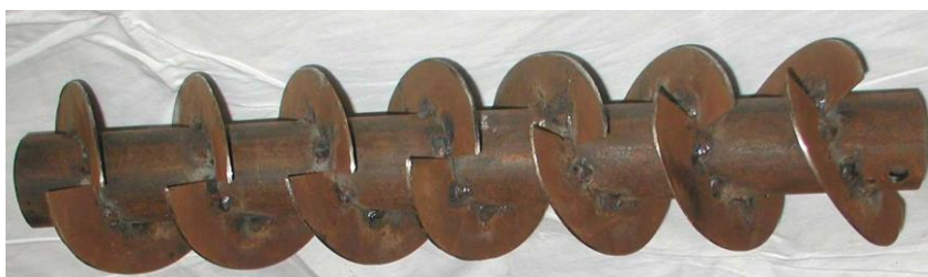
Fig. 2 – General view of the working body, made in the form of a shaft with inclined flat blades
