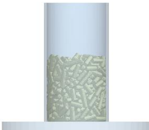
Fig. 3 -Experiment on simulated angle of repose of cotton straw
