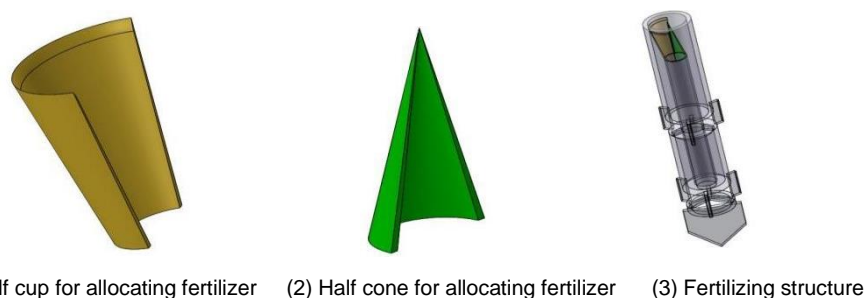
Fig. 4 - Composition of fertilizing unit
