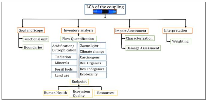
Figure 2. LCA of the coupling and its environmental effects.
