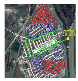
Figure 8. Unusable portion of pipe network (red) and selected section for temporary supply (green). Blue trace lines are the identified segments to be closed off.
